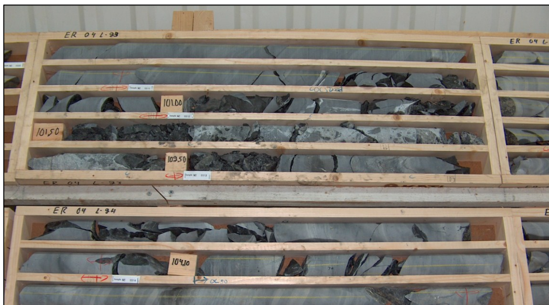
Figure 20-4: ER04 core photo illustrating a zone of intense fracturing
